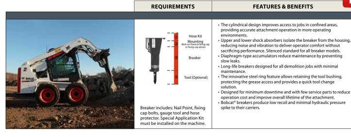
**Description:** Bobcat<sup>®</sup> breakers offer high performance, low maintenance, and are easy to use. All breakers feature a frame with a cylindrical design, providing improved access to jobs in confined areas. All breakers have a silenced housing as standard.
