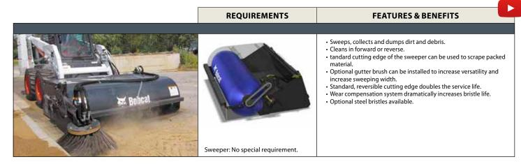
Description: This handy attachment sweeps, collects and dumps dirt and debris. In addition, it cleans up in forward or reverse. Perfect for cleaning parking lots, sidewalks, docks and warehouses. It can also be used to spread material evenly across a site. An optional gutter brush is available.
